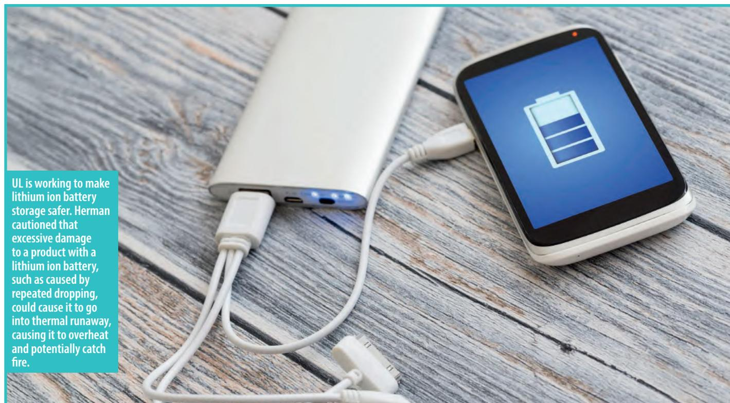
UL is working to make lithium ion battery storage safer. Herman cautioned that excessive damage to a product with a lithium ion battery, such as caused by repeated dropping, could cause it to go into thermal runaway, causing it to overheat and potentially catch fire.
