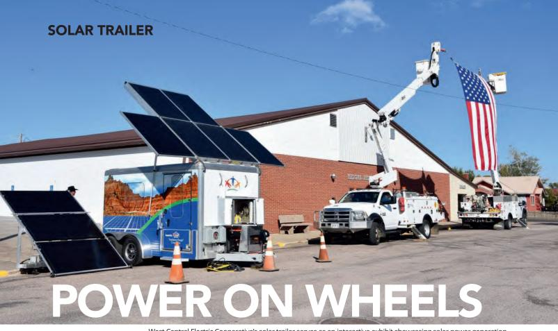
West Central Electric Cooperative's solar trailer serves as an interactive exhibit showcasing solar power generation in action for members. Equipped with a built-in generator, battery storage unit, inverter, and six rooftop solar arrays, the trailer is a great resource for public outreach and education efforts in South Dakota.
